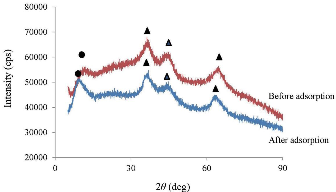
**Fig. S1.** XRD Patterns of NA12 Before and After Adsorption of Phosphate Ion
