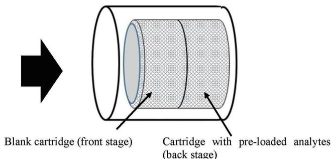
Fig. 2. Recovery Test Using a Connection Assembly for an AERO Dual Cartridge Holder
