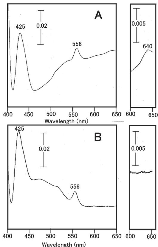
**Fig. 5.** Comparison of Reduced Minus Oxidized Difference Spectra for the Inactivation of Membrane Vesicles Irradiated with 405-nm Blue Light at an Irradiance of a 20 mW/cm<sup>2</sup> for 3 min (Energy Density: 3.6 J/cm<sup>2</sup>) (4.8 mg/mL, B), as Compared with Control Reduced Minus Oxidized Difference Spectra for Non-Irradiated Vesicles (2.4 mg/mL, A)
