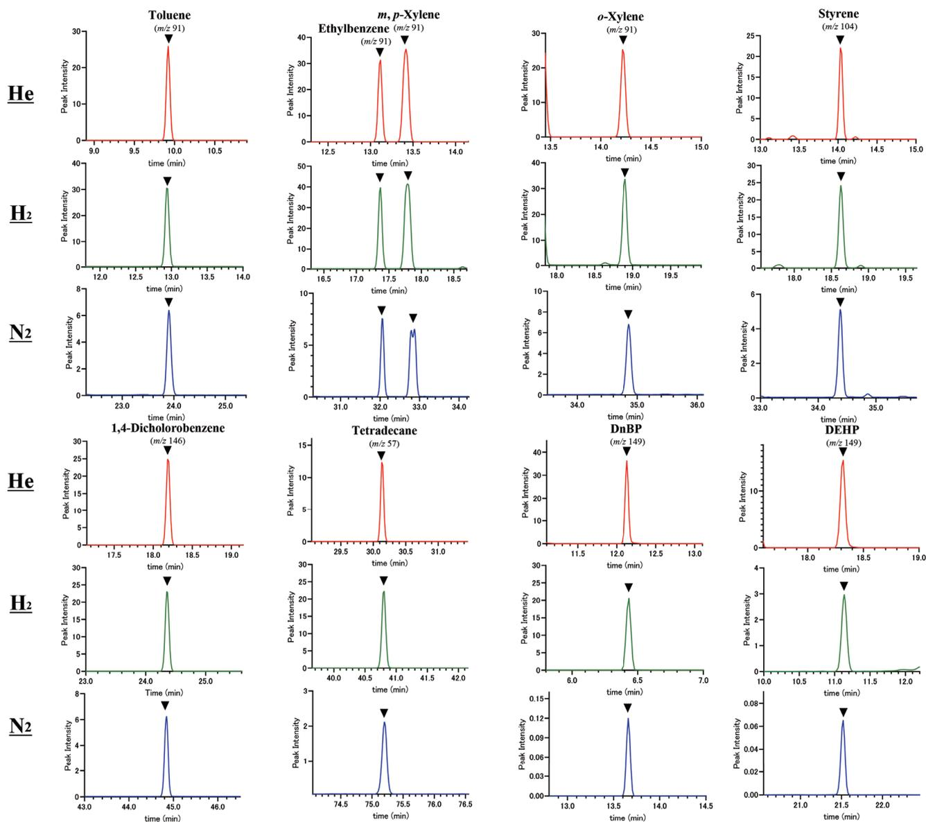
Fig. 2. SIM Chromatograms of the Target Chemicals for Each Carrier Gas
